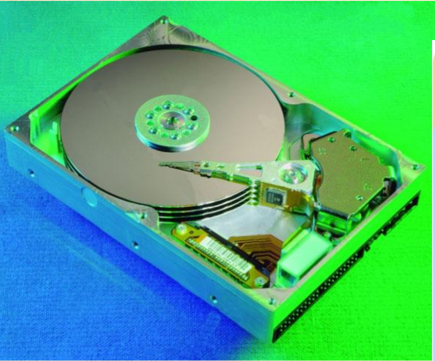
Exhibit 2-12 How data is stored on magnetic disks
