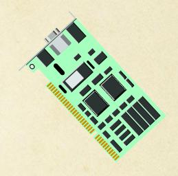
Plug and Play – computer automatically configures the adapter card when it is installed.
