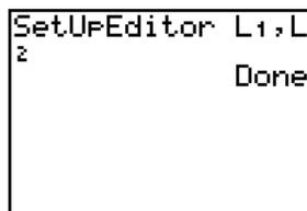
The second is to manually enter a particular list name. In the STAT EDIT screen, move the cursor over the list names, then arrow to the right until you reach a blank list.
